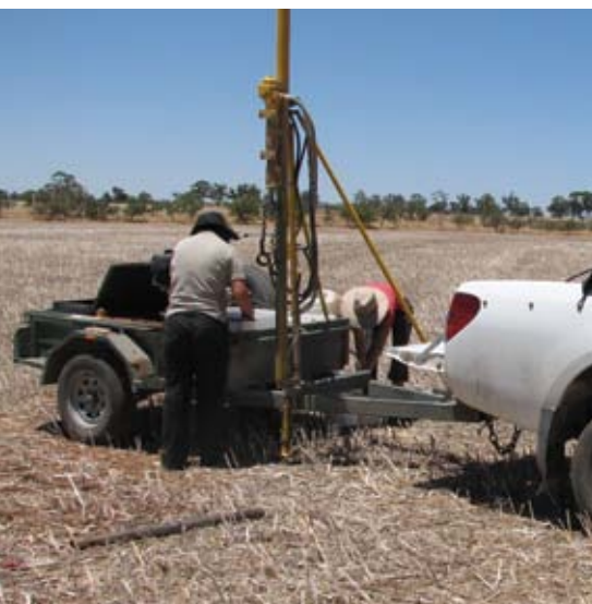
Field sampling of soil cores. Left: trailer-mounted soil corers (Photo: L Macdonald, CSIRO). Middle: a soil core sample (Photo: Josh Tefler, Rural Solutions SA). Right: A magnified image of charred organic carbon fragments.
