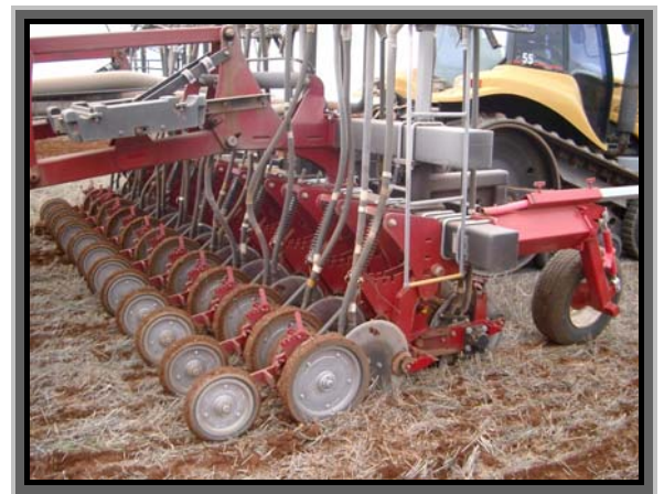
Close up of the working mechanisms of a no-till disc seeder. (Photo: SANTFA)
